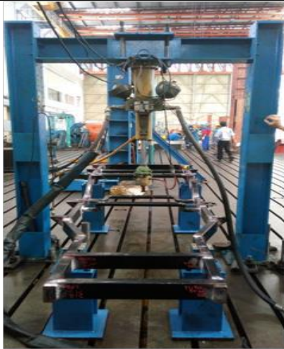
Fig.11: Bending test on welded chassis
