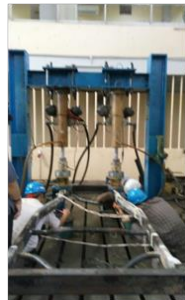
Fig.16: Torque test on bent chassis
