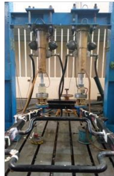
Fig.15: Torque test on welded chassis
