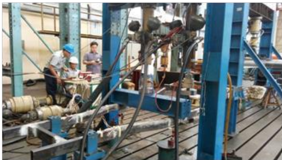
Fig.12: Bending test on bent chassis
